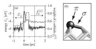
Fig. 2. (a) Elementary reconstruction process with the one-electron energy  $\varepsilon_i$  and the weight on s orbitals  $f_s^{(i)}$ . (b) An asymmetric dimer on a resultant crack. The black rod and black ball correspond to the ' $\sigma$ ' and ' $\pi$ ' states, respectively.
