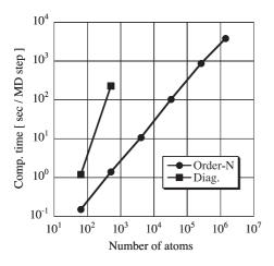
Fig. 1. Computational time for bulk silicon as a function of the number of atoms, up to 1423909 atoms. The CPU time is measured for one time step in the molecular dynamics (MD) simulation. A tight-binding Hamiltonian is used with the perturbative order-*N* method and the exact diagonalization method. We use a standard workstation with a single CPU and 2 GB of RAM.
