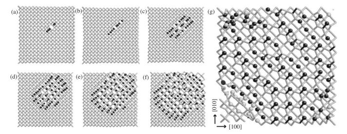
Fig. 3. Snapshots of a fracture process in the (001) plane. The sample size is  $n_{100} \times n_{010} \times n_{001} = 33 \times 33 \times 33$  (4501 atoms). The time interval between two successive snapshots is 0.3 ps, except that between (f) and (g) (approximately 1.3 ps). A set of connected black rod and black ball corresponds to an asymmetric dimer, as in Fig. 2(b). The lower left area has not yet been fractured.
